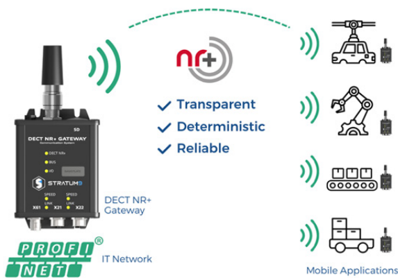
The NR+ Gateway enables wireless, unmodified PROFINET/PROFISAFE transmission to mobile applications.
