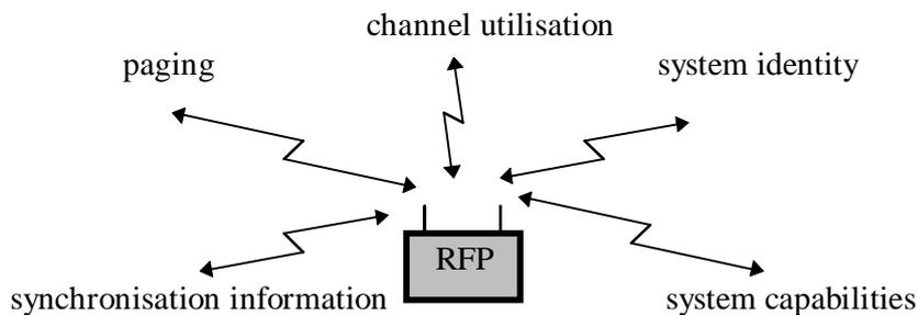
Figure 5. The DECT fixed part beacon function
