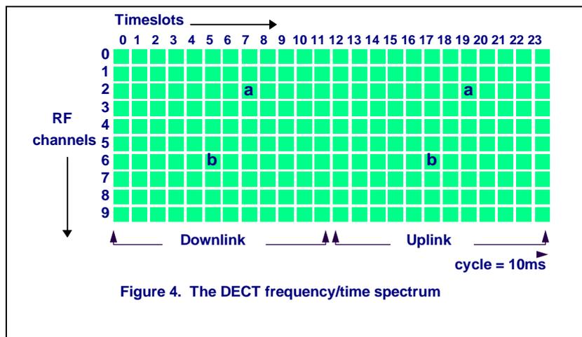
Figure 4. The DECT frequency/time spectrum
